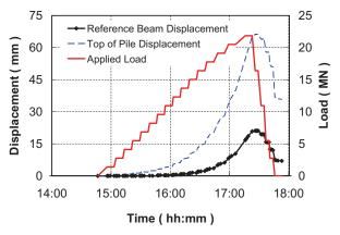
[FIG. 6] Reference Beam Displacement Compared with Applied Load (LOADTEST Project Reference No. 620, 2004)
