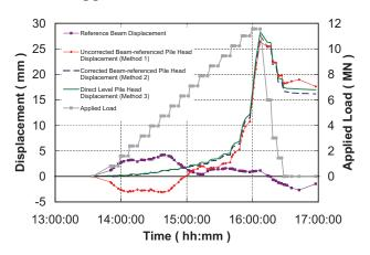
[FIG. 8] Direct Comparison of Results of Method 2 and Method 3 (LOADTEST Project Reference No. 539, 2005)
