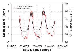
[FIG. 7] Shaded Reference Beam Displacement Compared with Temperature Variation (LOADTEST Project Reference No. 213-3, 2005)
