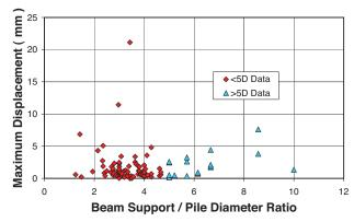
[FIG. 3] Maximum Reference Beam Displacement vs. Support/Diameter Ratio (LOADTEST Database, 1995-2004)
