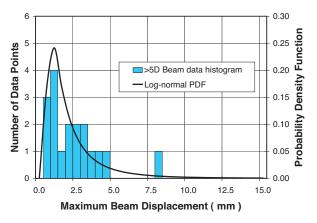
[FIG. 5] Probability Density Function (PDF) of Max. Beam Displacement (>5D Subset) (LOADTEST Database, 1995-2004)
