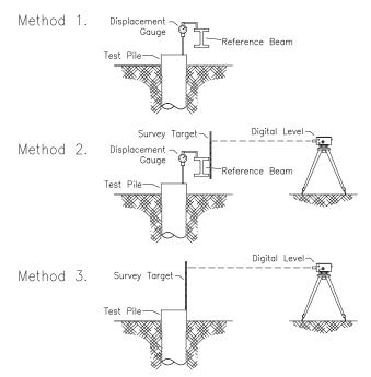
[FIG. I] Schematics of Pile Head Displacement Measurement Methods
